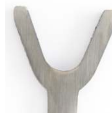
Unretouched photograph of a section cut from a flame- hardened McKissick sheave (etched 2-1/2 minutes)
