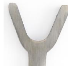
Unretouched photograph of a section cut from a flame- hardened McKissick sheave (etched 2-1/2 minutes)
